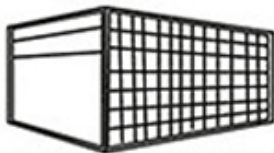
LD-9/Type 5 Full Width Lower Deck Container
