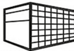
M-1/Type 2 Main Deck Pallet Container
